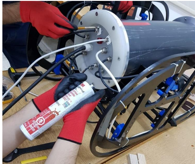
Figure 6-7 Applying chemical isolation
